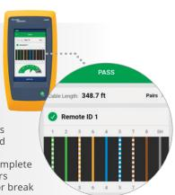
LinkIQ<sup>™</sup> validates cable performance via frequency-based measurements
